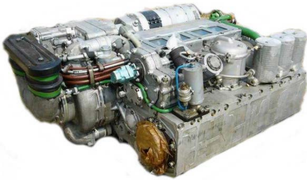
Figure 1. Compact 6TD diesel produced by Kharkiv Malyshev Factory in Ukraine
